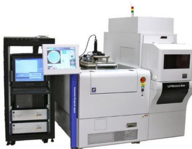
ISI can set up their testing with EG, TEL, and Accretech Probers (shown above) and they can configure for virtually any other prober. Their electronics and test software are independent from the wafer prober and their test head can be installed on any prober. A simple cantilevered probe card can be used to provide multi-device testing capability on 200 or 300 mm wafers.
